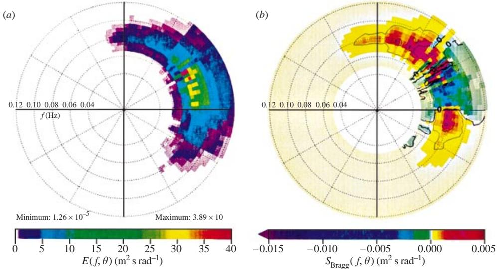
FIGURE 11. (a) Predicted wave spectrum  $E$  in region  $S_1$  (figure 8) and (b) corresponding Bragg scattering source term  $S_{\text{Bragg}}$ , based on bottom spectrum  $F_1^B$ . Contours in (b) are solid for positive values (yellow to red colour shades), solid and thick for zero, and dashed for negative values (green to blue colour shades).  $H_s = 0.92$  m;  $f_p = 0.078$  Hz; mean direction at  $f_p = 69.5^\circ$ ; spread at  $f_p = 24.00^\circ$ .
