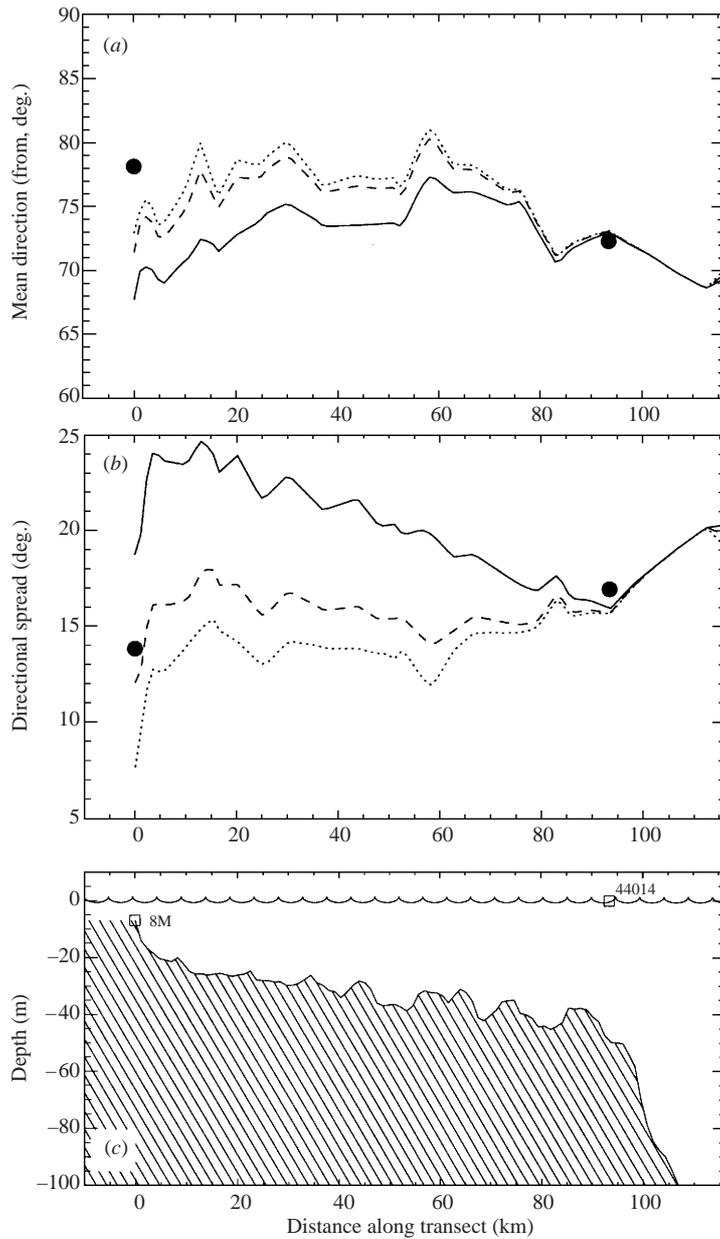
FIGURE 12. Measured (●) and predicted (—, with Bragg scattering using  $F_1^B(I)$ ; ---, with Bragg scattering using  $F_2^B(I)$ ; ···, without Bragg scattering) variations of (a)  $\bar{\theta}$  and (b)  $\sigma_\theta$  at the peak frequency  $f_p$ . Results are shown for 20 October 2000, at 21:00 GMT, along a cross-shelf transect (c) extending from the 8 m depth array to deep water offshore of NDBC buoy 44014. A maximum value of  $k/l = 5$  was used in the scattering calculations.
