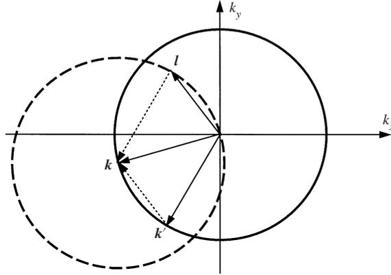
FIGURE 1. Geometric properties of wavenumbers satisfying the resonance condition. The interaction between a surface wave with wavenumber  $k'$  and a bottom component with wavenumber  $l$  excites a surface wave with the sum wavenumber  $k = k' + l$ . For fixed  $k$ , the resonant  $k'$  and  $l$  lie on the solid and dashed circles, respectively.
