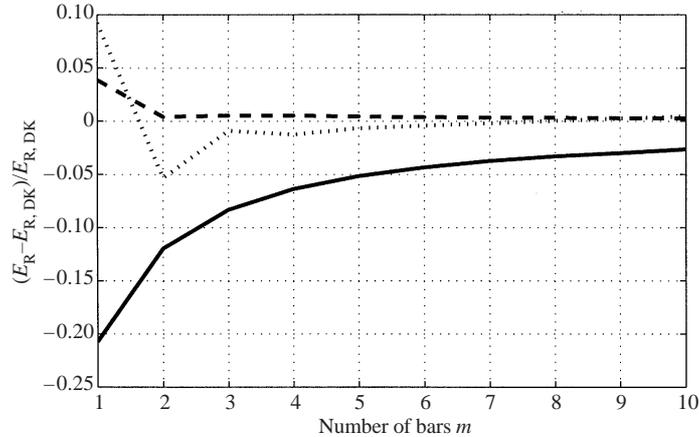
FIGURE 7. Relative differences between the reflected energy predicted by the stochastic theory (equation (3.8)) and the spectral form (equation (3.12), replacing  $\kappa_{DH}$  by  $\kappa_{DK}$ ) of Dalrymple and Kirby's theory, as a function of the number of bars  $m$ . All other parameters are the same as in figure 6. The incident wave spectrum is shown in figure 6.
